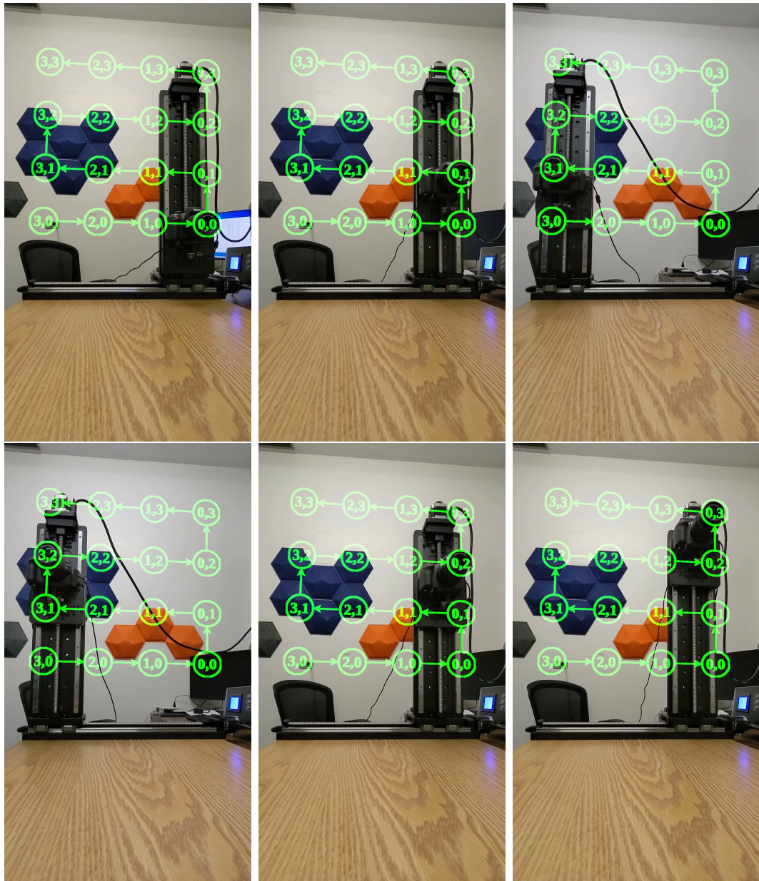
Figure 3.3: Camera system capture movement pattern for a 4 \times 4 set of images. Points and movement pattern are drawn on the photos. Each point has its own co-ordinates that are saved for each image.
